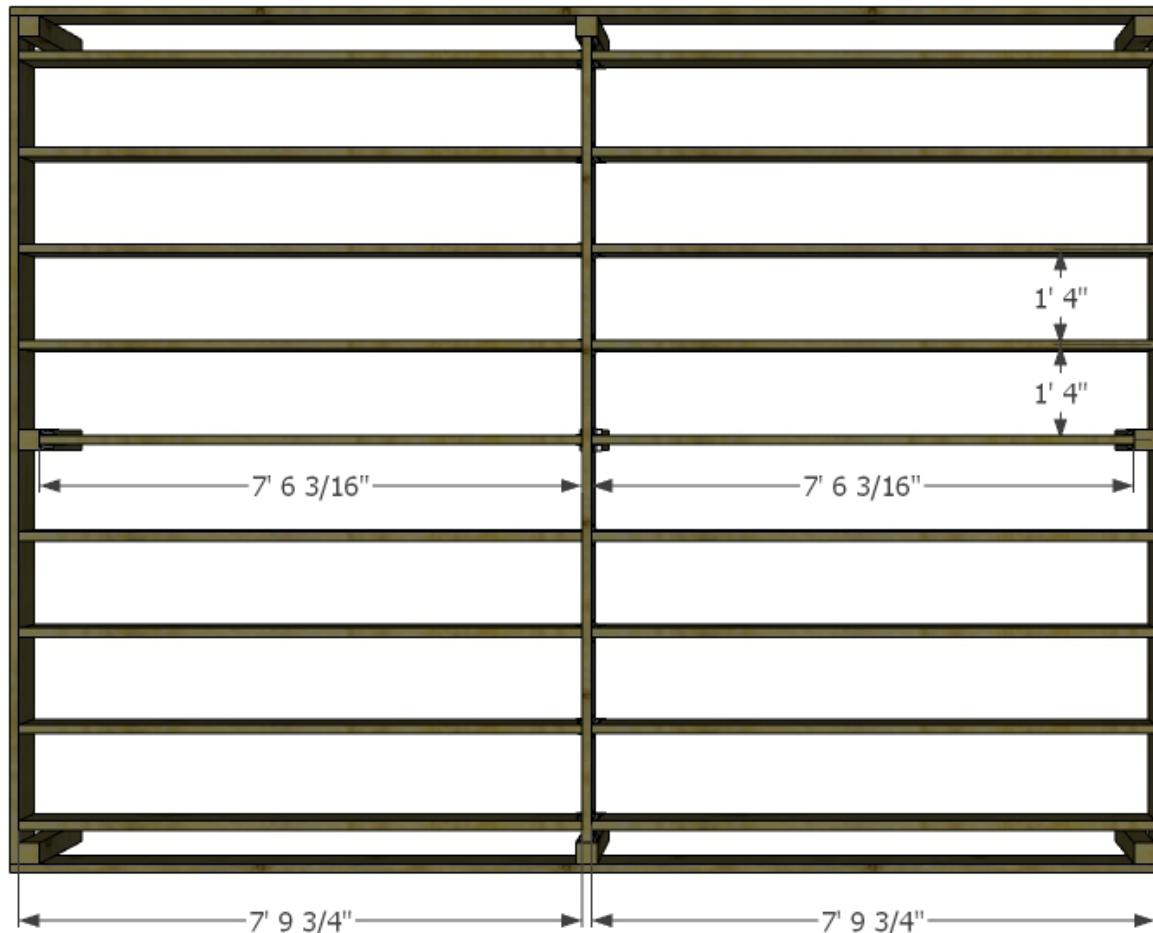
Locate the joist spacing by finding the center of short center beam
